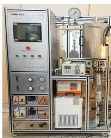
Plate I: MicroActivity Reactor (MAT) for Testing Zeolites and other Catalysts
