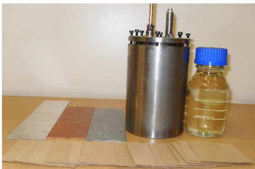
Figure 11: Bespoke Ageing Test Vessel with ageing components
