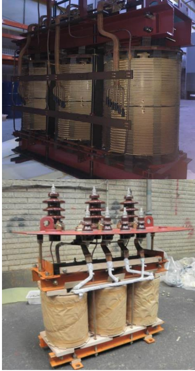
Figure 3: The inside of a transformer with solid insulation
