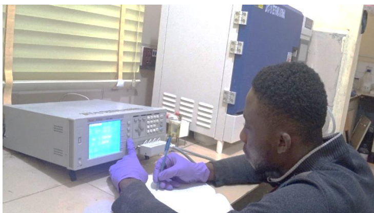
Figure 18: A Postgraduate student using LCR Bridge for dielectric measurement
