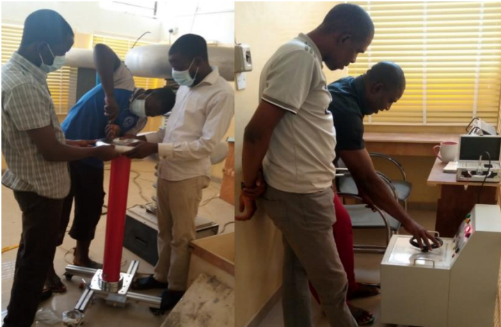
Figure 16: Installation and testing of the 100 kV HVAC system
