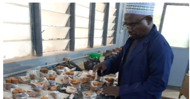
Cored specimens for unconfined compression test by Garba Alhaji Murtala, a doctoral candidate under the group
