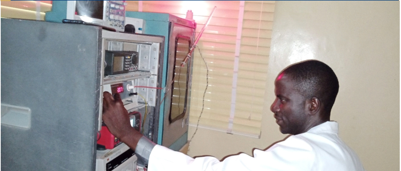
Dr. Abdulsalam I. Galadima working with the 35 kV HVDC experimental set-up for oil breakdown test
