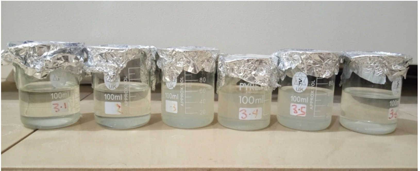
Prepared natural ester nanofluids in the laboratory
