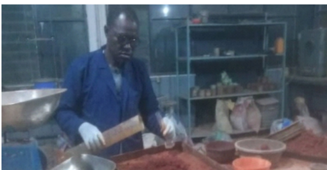
Preparation of sample of unconfined compression test by Ashiru M. Ashiru a doctoral candidate under the group
