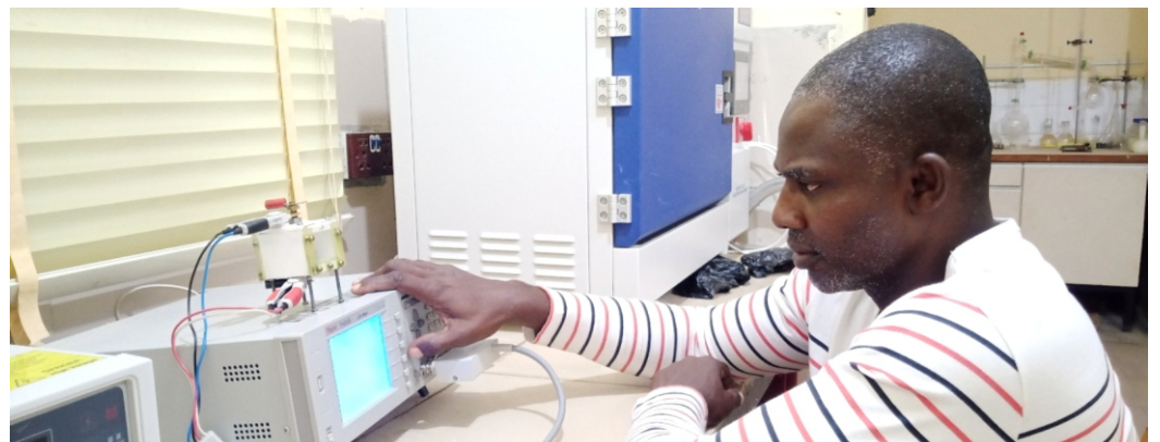
Prof. Abdelghaffar Amoka Abdelmalik doing dielectric measurement of polymer samples with LCR Bridge test
