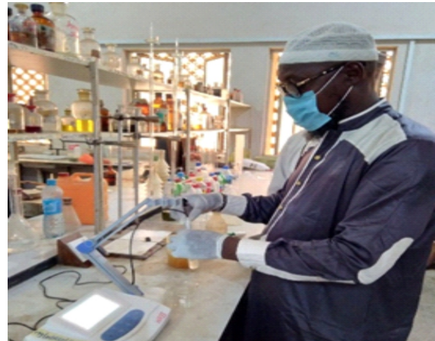
Urease activity determination through electrical conductivity test by Garba Alhaji Murtala
